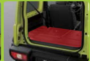
The back seats and luggage room floor are coated with plastic for easy dirt/stain removal.
