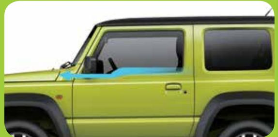
Dipping front door window lines expand visibility through the window.
